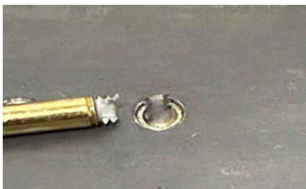
1/4"-20 Insert in A36 Material, Bolt Failure After bolt failure, the remaining bolt segment was removed by hand, with no insert thread deformation.
