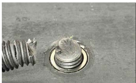
3/4"-10 Insert in A36 Material, Bolt Failure After bolt failure, the remaining bolt segment was removed by hand, with no insert thread deformation.
