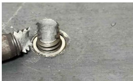
1/2"-13 Insert in A36 Material, Bolt Failure After bolt failure, the remaining bolt segment was removed by hand, with no insert thread deformation.
