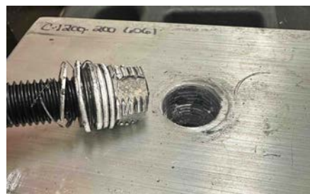
3/4"-10 Insert in 6061-T6511 Material, Insert Failure due to Substrate Material
